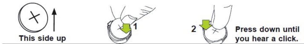
Figure 17. Install the battery
